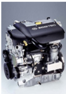
The Opel 2.0 DTI 16V engine, 1996.
