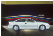
Wind-tunnel testing of the Opel Calibra, 1989.
