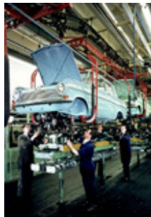
Final assembly (wedding) of an Opel Kadett A in the Bochum plant, 1963.
