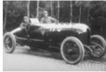
Carl Jörns at the wheel of a 260 hp, 12.3-liter Opel race car from 1914. Beside him is his navigator, Kurt C. Volkhart..
