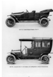
The two variants of the 10/24 hp Opel from 1911: a torpedo double phaeton and a covered limousine with a fold-down windshield.
