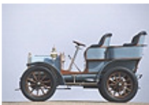
The two-cylinder, 10/12 hp Opel Motor Car, the first model built entirely by Opel.
